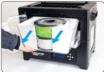
9. Take the lid together with two rolls of filament out from the printer.
